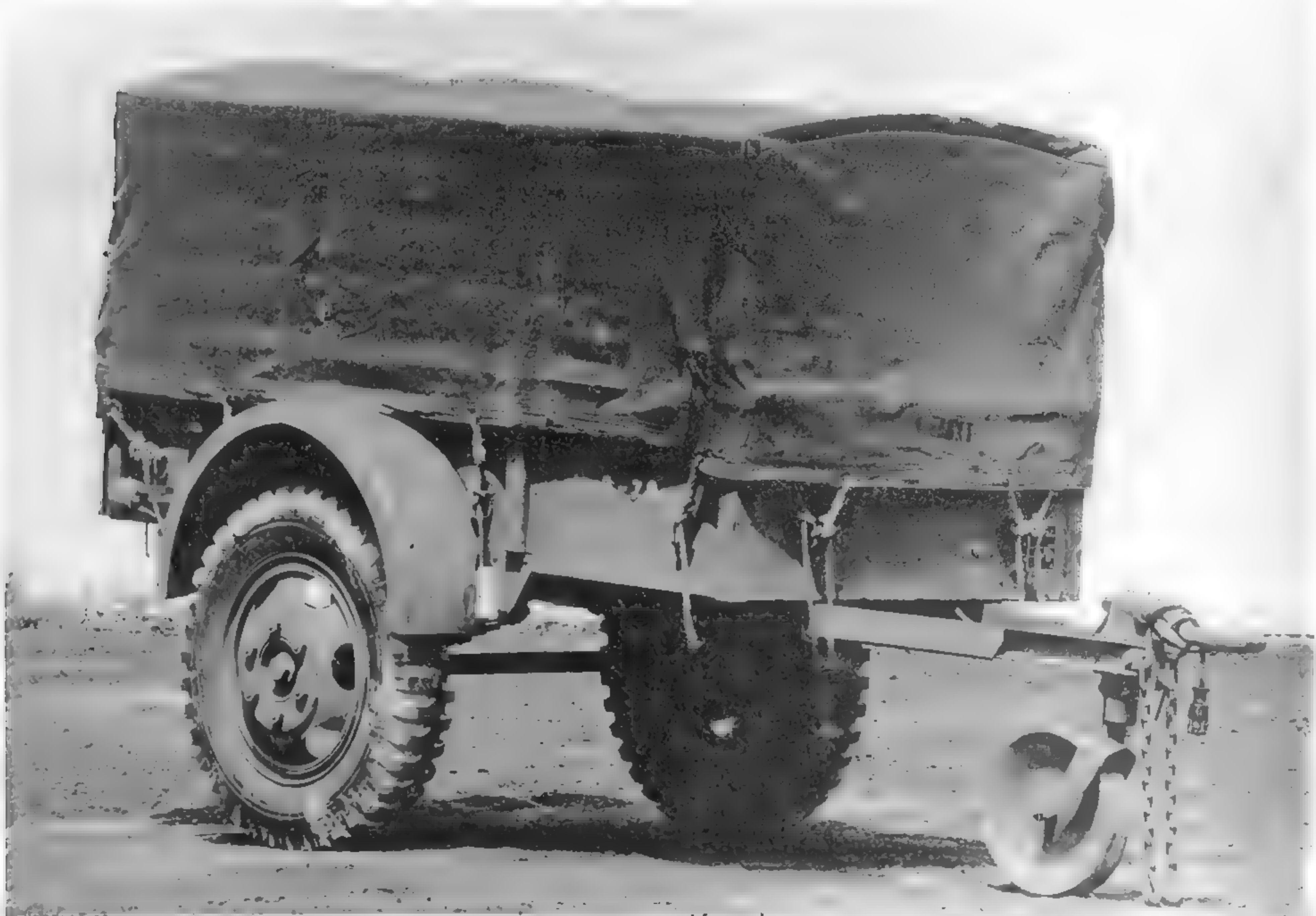
This trailer built by Hobbs and is representative of the all-steel 1-ton trailers produced toward the end of WWII. (U.S. Army photo)
